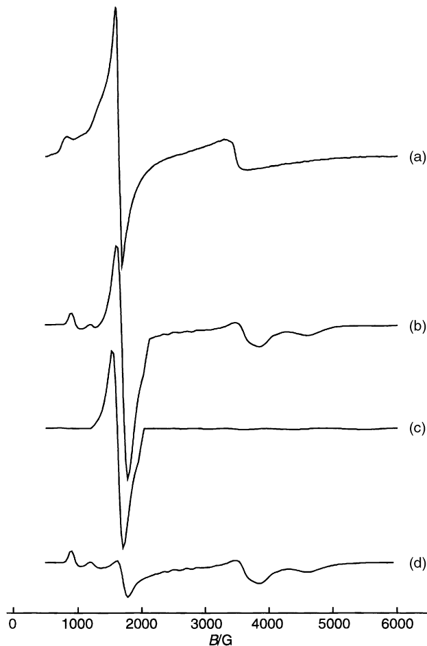
Fig. 14 (a) Powder EPR spectrum of complex 4 obtained in the X-band at 80 K. (b) The total simulated spectrum as a sum of the spectra (c) and (d), assuming S = 5/2 .
